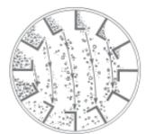
Backside wear on drum flighting due to veiling action
