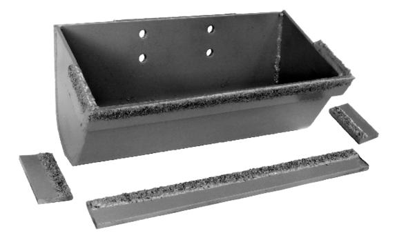
Kenco Engineering elevator buckets with Tungsten Carbide Impregnated (TCI) wear lips provide substantially longer wearlife than standard buckets. A feature unique to Kenco buckets is the TCI "cleanup" lip. These wear lips project 1/2 inch farther than normal to help prevent material from accumulating and hardening at the bottom of the elevator.
