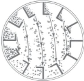
Backside wear on drum fighting due to veiling action
