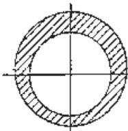
cross section view of Kenco elbow casting showing 50% thicker wall at outer radius
