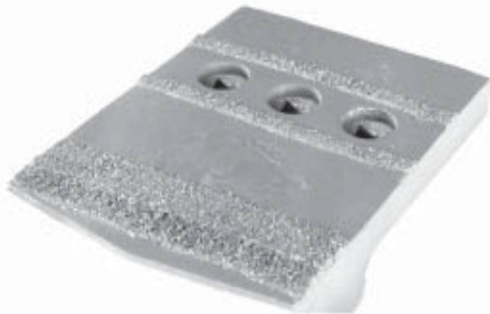
KENCO Engineering *Half-Arrow* Segments provide the ultimate in moldboard protection and bucket lip penetration. Designed for use on rock buckets, *Half-Arrow* Segments virtually eliminate moldboard wear between teeth. And the beveled, pointed leading edges create excellent penetration of shot rock and other aggregate material.
